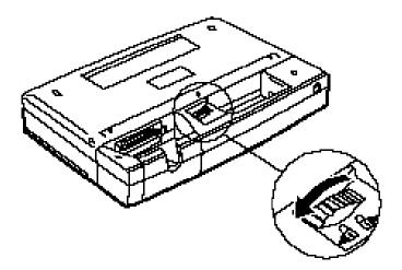
5. Disconnect the battery case from the printer.
